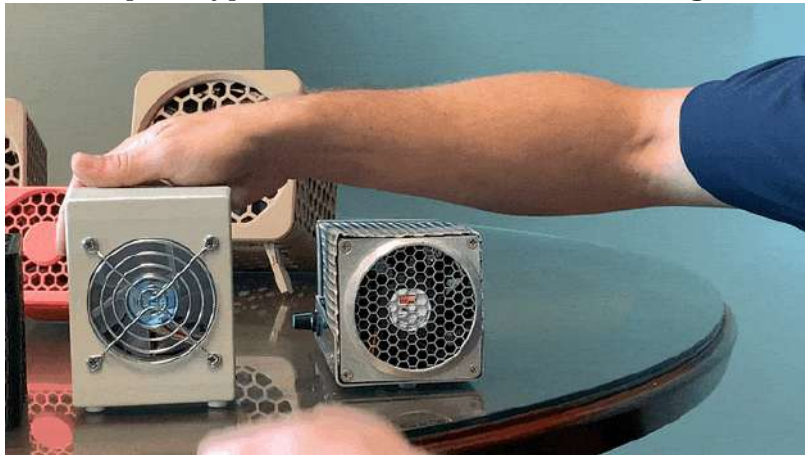
Our second prototype made with an off the shelf plastic case
