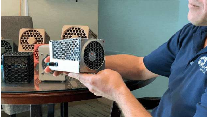
Our first prototype with a handmade metal housing
